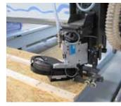
The battens are fixed to the sheathing using the BeA Autotec jumbo coil nailer for wire collated roundhead nails. The tool can handle nails ranging from 45 – 70 mm in length. Depending on the nail diameter, the magazine can hold up to 1,000 nails. The jumbo coil magazine is simply loaded from above.
