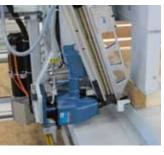
BeA Autotec strip nailers for roundhead nails up to 160 mm in length are used to join the framework. The long magazines of the BeA Autotec strip nailers can be simply and easily loaded from above.
